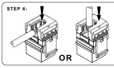
Place cap on jack and press to make sure it is fully seated. The cap opening allows the cable to enter the jack from side to rear.
