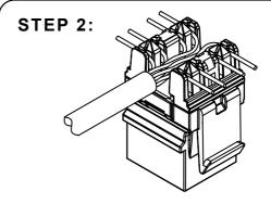
Press the wires through the projecting portion of terminals until fixed.
