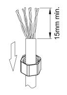
Put cable through the Nut. (OD: 4~6mm; 23~26 AWG) Strip the cable for minimum 15mm.
