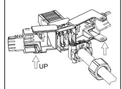
Put the cap on the IDC tower. The arrows on the jack and the cap should face the same direction. Put the cap into position.
