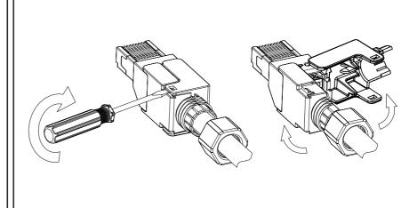
Insert the slotted screwdriver into the slot and rotate to open the jaws
