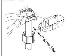
Cut the excess wires off. The tips of the wires should protrude no more than 0.5mm
