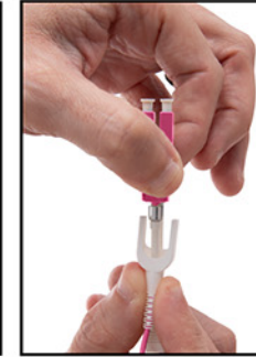
6. PUSH BOOT ON TO CONNECTOR
