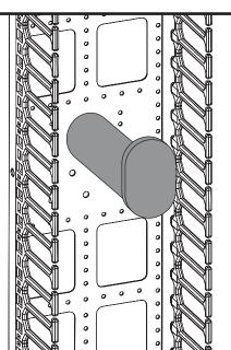
1. Locate the 3 sets of (3) 6mm dia. holes in a triangular pattern as shown.
