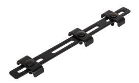
The Bar Splice Kit provides additional strength when joining two basket trays on a horizontal plane. Each kit includes one straight bar splice and 3 sets of M6x20 carriage bolts, M6 nuts, and top splice washers.
